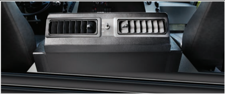
A high performance tunnel mount HVAC unit is standard on the 3000 Model and is available as an option on the 4000 Model.
