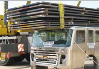
120,000 lb. Crush Test
